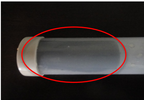
Figure 1. The driver installed in one end of the tube.
